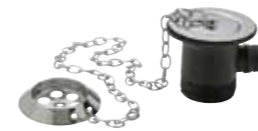
1 1/2" BSP bath waste & overflow, brass flange, with parking plug & oval link chain
