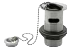
1 1/4" BSP brass vanity waste & overflow with rubber plug & ball chain
